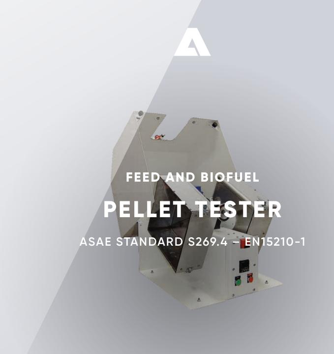
The ANDRITZ pellet tester is used for testing of pellet quality and durability. The method is approved according to the international ASAE Standard S269.4 – EN15210-1.
