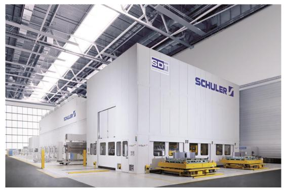
One of the largest orders in Schuler's 175-year history was received from FAW Volkswagen Automotive, China. The order comprises three press lines with ServoDirect technology. The servo-press lines are used mainly to produce car body parts, such as hoods or doors.
