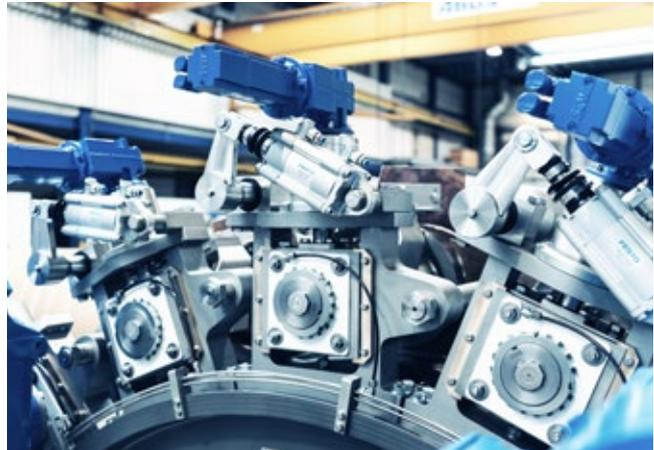
Smart adjustment control of the applicator rolls
