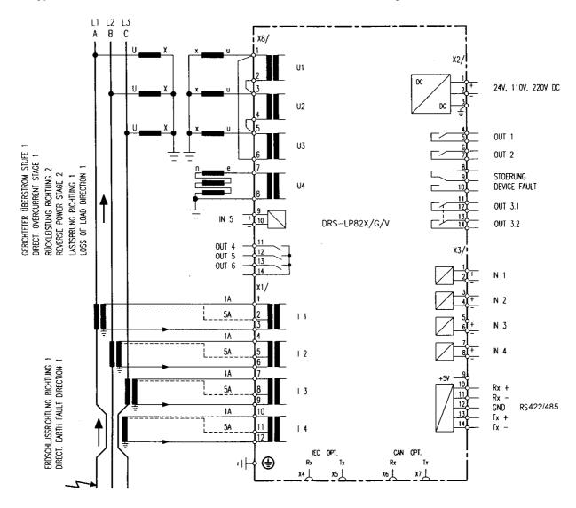
If the unit decoupling relay is connected in this form and the increasing active power supply (Generator down, mains up) the setting parameter of the unit decoupling relay "directional power" = direction 1 is to set.
