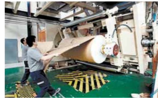
▲ A new roll of paper is being loaded into the ANDRITZ BMB coating system, which is followed by online calendering on the ANDRITZ Küsters equipment.
