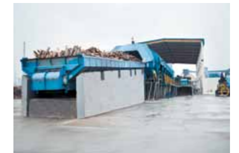
▲ The mill's fiber supply is principally softwood (masson pine and fir), but it can also produce bleached hardwood as well (above). The Huaihua mill boasts the first horizontally-fed HHQ-Chipper™ in China (upper right). Logs being loaded into the ANDRITZ debarking drum. Capacity for the debarking/chipping line is for 350 m³ sob/h (lower right). ►
