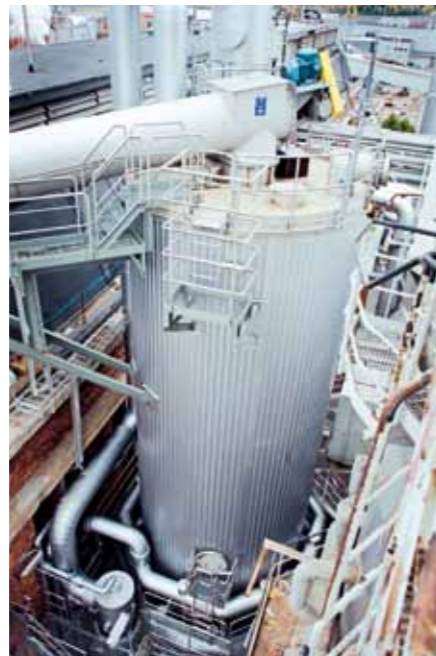
▲ The bottleneck in the Varkaus mill's fiberline was the chip feeding system. In November 2007, ANDRITZ installed a Diamondback® chip bin and TurboFeed® chip feeding system, "January and February of 2008 were two of our best months for production since I have been at this mill," Varis says. "Normally, the winter months are very difficult for us, but the improved chip quality and the new feeding system have been excellent."
