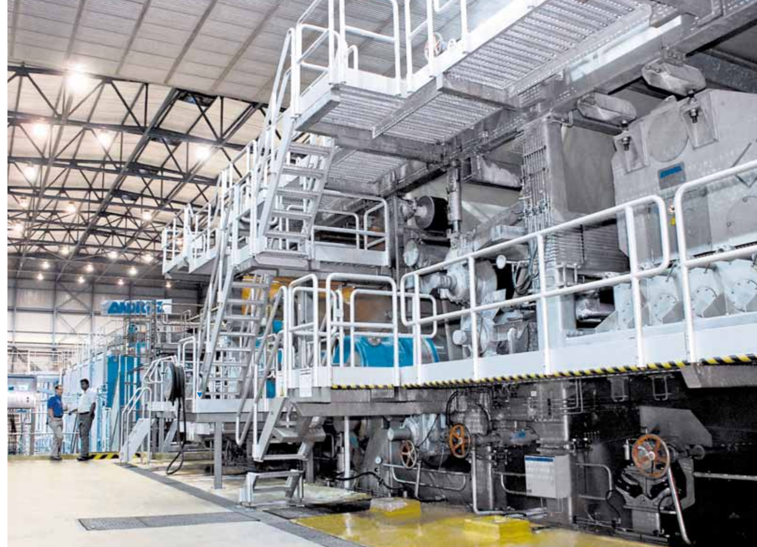
▲ ANDRITZ delivered a turnkey pulp drying line which includes the approach flow system, pulp machine, airborne sheet dryer, densification press, cutter/layboy, and automated baling line. The pulp machine (above) features twin wire forming technology and a PrimePress X shoe press.
