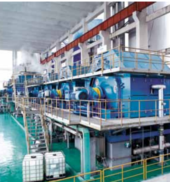
The fiberline at Huaihua is one of the largest in China. A total of six DD Washers are employed for washing, oxygen delignification, and ECF bleaching (left). Part of the oxygen stage and bleaching line. Bleached capacity is 1242 admt/d on softwood and 1358 admt/d on hardwood (right). ▼
