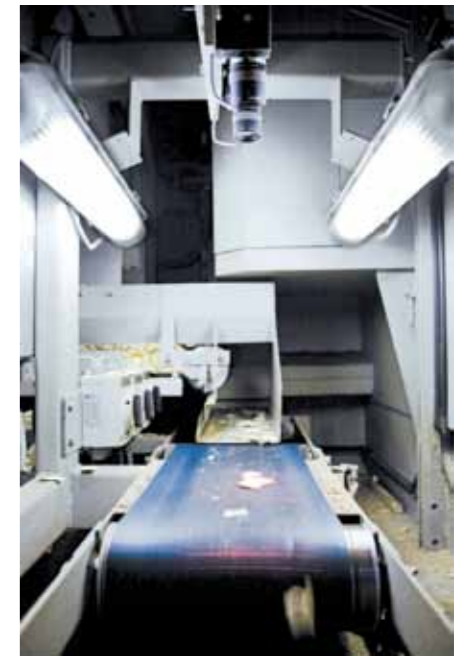
▲ The ChipScan™ online analyzer gives operators accurate data on chip length, thickness, and variability in real-time.
