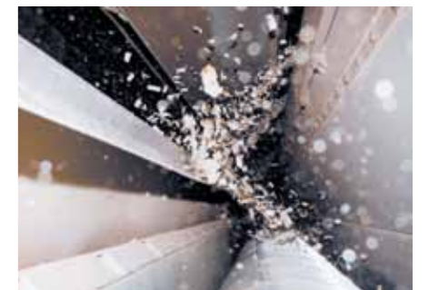
▲ The JetScreen™ thickness screen makes it easy to optimize chip quality for the digester. Chip quality is adjusted simply by adjusting the air pressure inside the unit.
