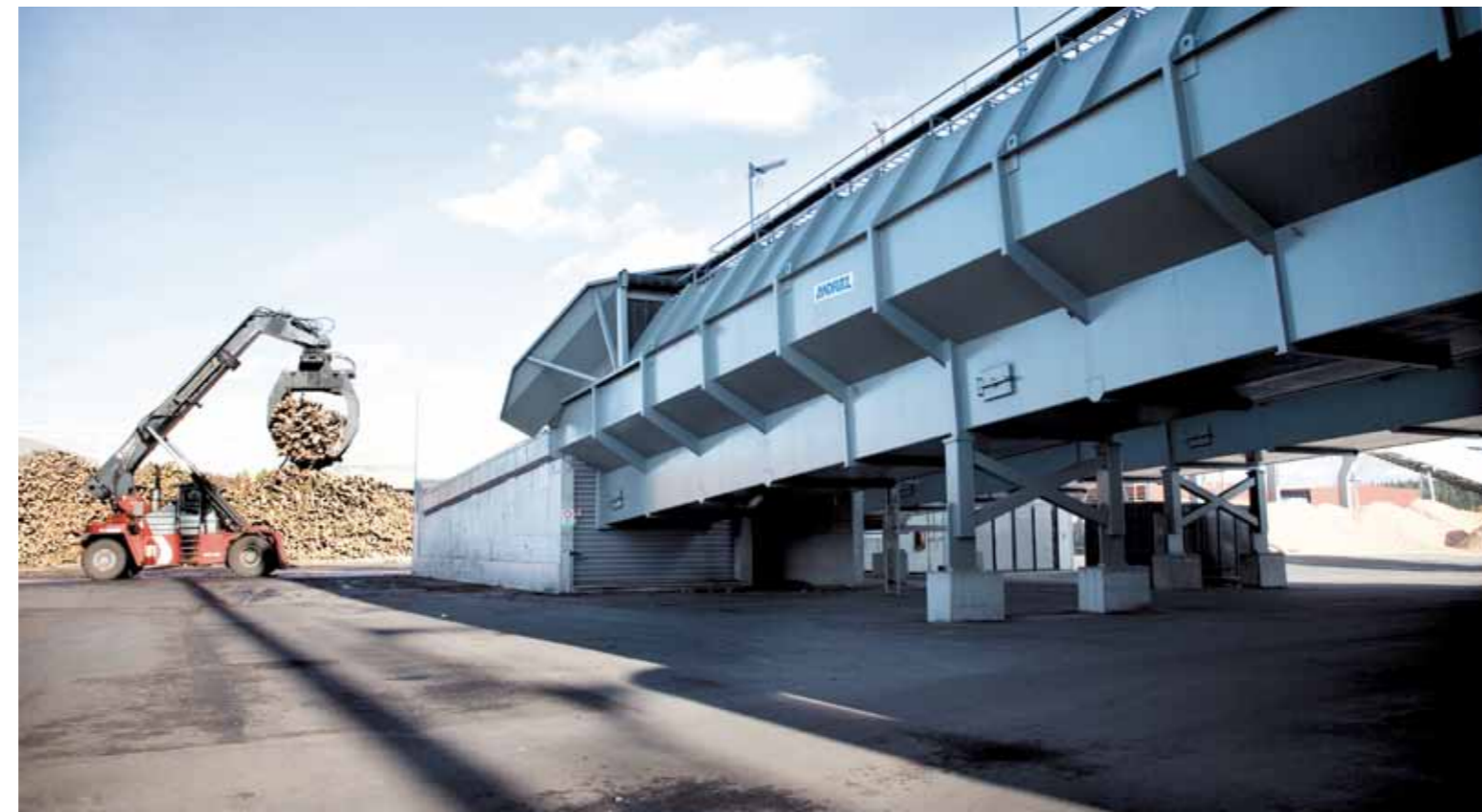
Logs being loaded into one of the PowerFeed™ infeed conveyors at Varkaus. The mill now has efficient de-icing with two temperature zones and the ability to load both long or short log bundles without bridging. ►
