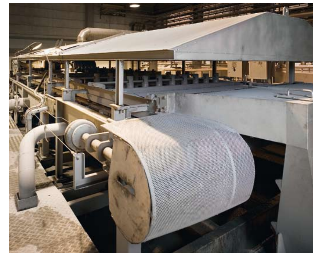
▼ The challenge: optimized dimensioning of existing equipment in order to handle changing sludge characteristics and to achieve higher dryness – using the same basic equipment. Andritz and mill personnel met the challenge by extending and upgrading the three existing gravity tables.
