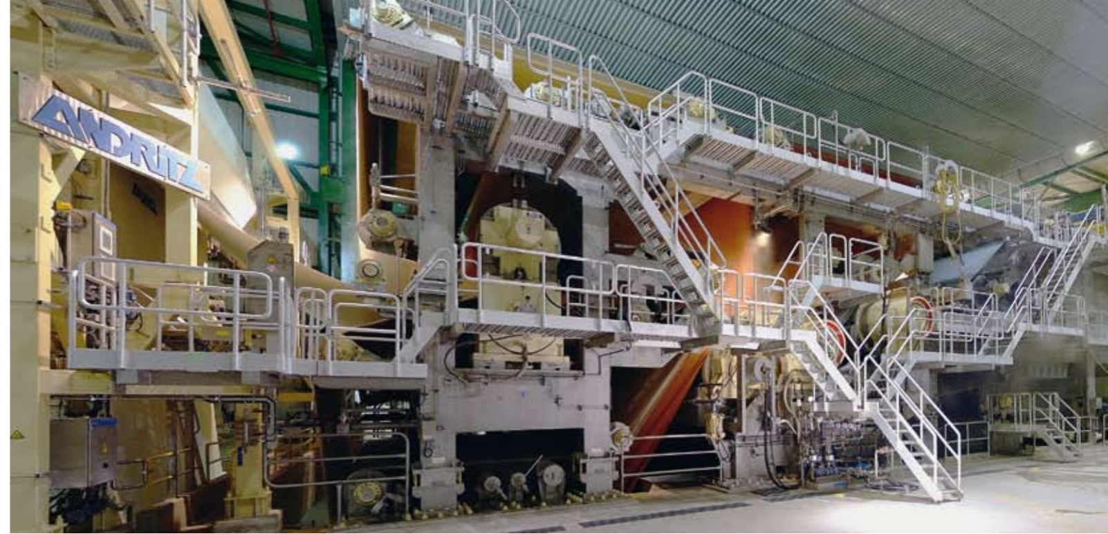
▲ The twin wire dewatering machine at CMPC. The addition of the shoe press helped Santa Fe overcome the poor drainage characteristics of the eucalyptus nitens , which comprise 70% of the furnish for Line 2.
