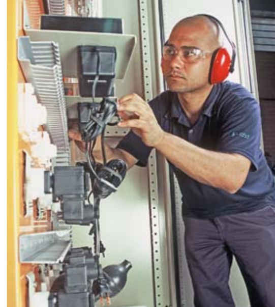
▲ A technician assembles an analyzer in the Sindus Andritz workshop. Sindus Andritz manufactures all kinds of devices for gas analysis, integrating the total system (sensor, sample handling, and system electronics).
