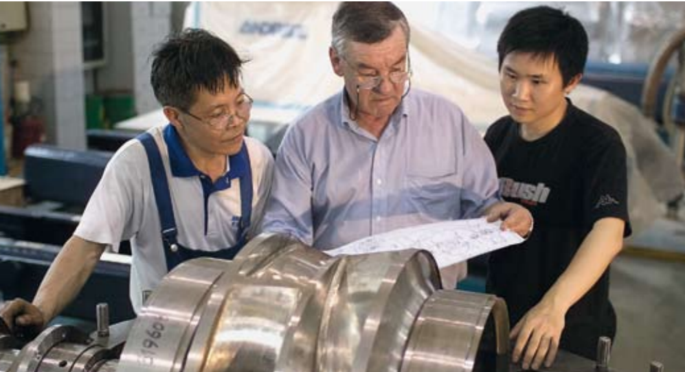
▲ Final inspection of a fan pump rotor. The same stringent quality control systems are in place in all of Andritz's facilities worldwide.
