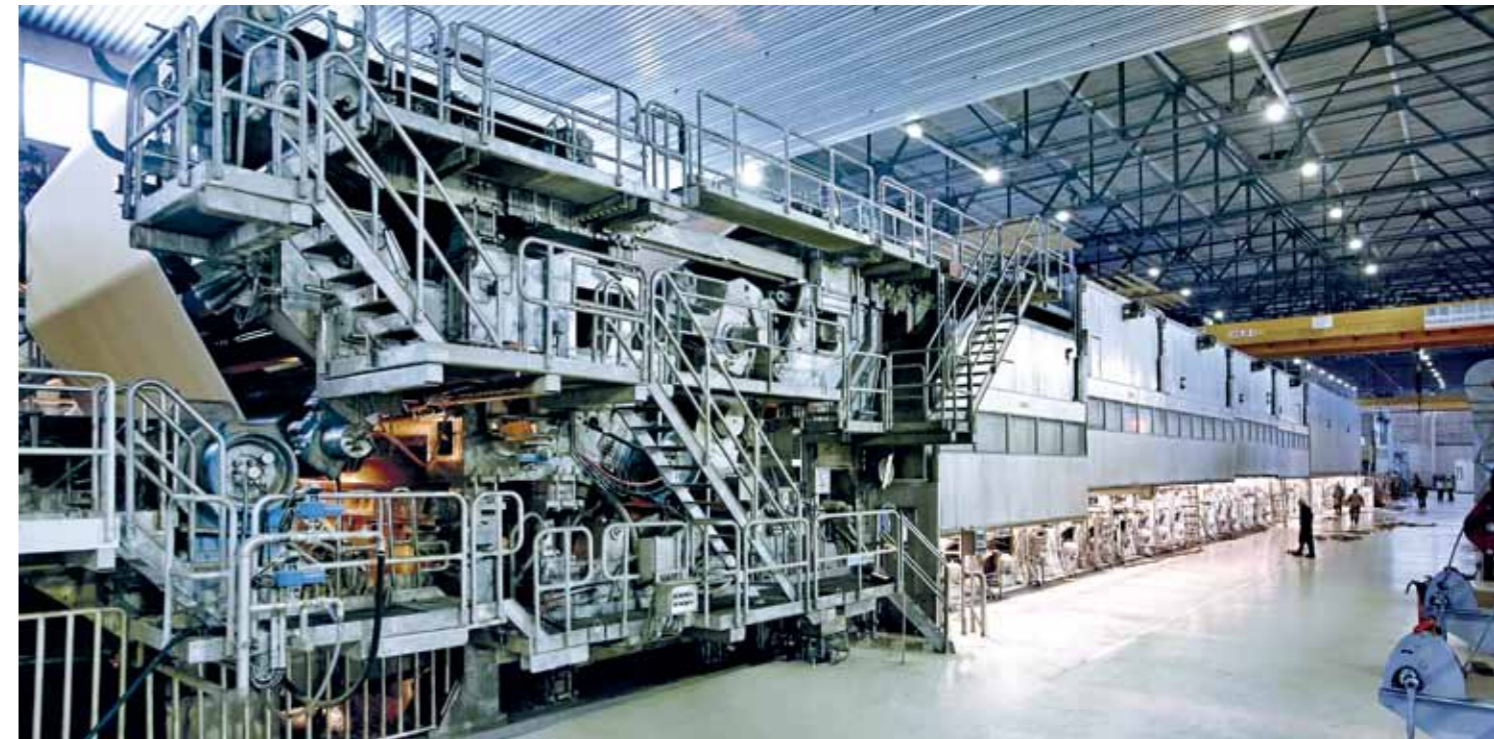
▲ PM originally came from Finland, where it produced machine-glazed kraft paper. ANDRITZ integrated parts of the old machine, including sections that required refurbishing and upgrading, with its own paper machine technology to deliver a state-of-the-art packaging machine.
