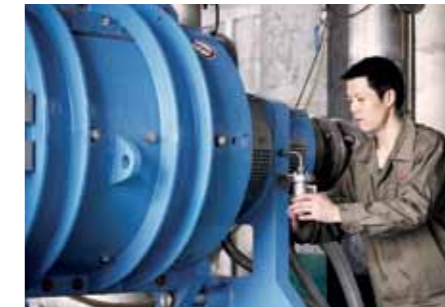
◀ Papillon stock prep refiners reduce energy costs and gently treat the fiber to ensure desired properties in the sheet.
