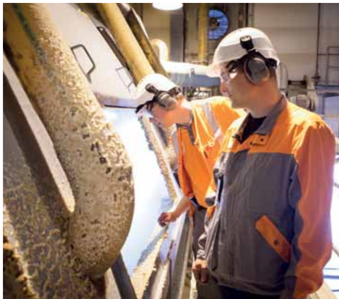
◀ Clean condensate from the Duct Stripper makes up most of the water for brownstock washing. Shown are Nikunen (foreground) and Peltonen at a wash press.
